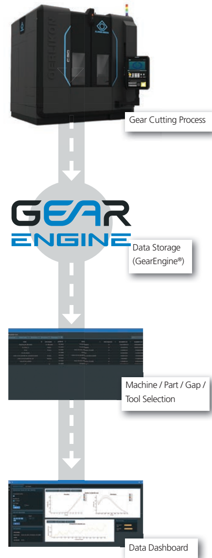
Fig. 1: Workflow of the Smart Process Control app based on machining data for an Oerlikon bevel gear cutting machine
